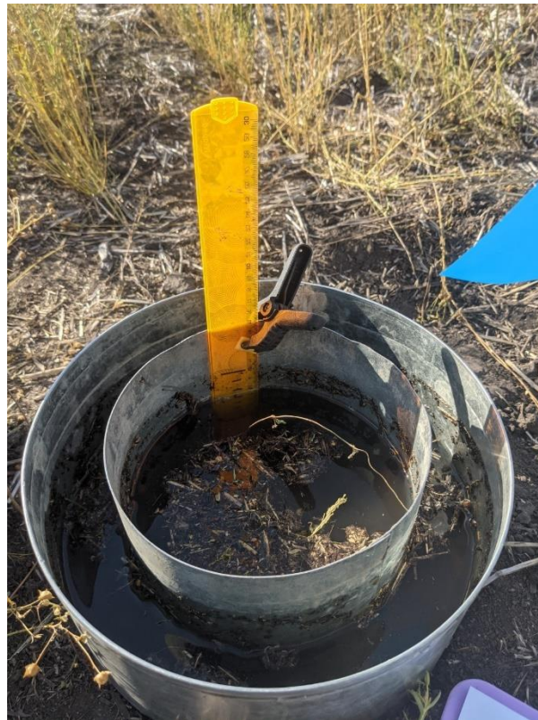
Figure 8. Double-ring infiltrometer used for water infiltration assessment.
