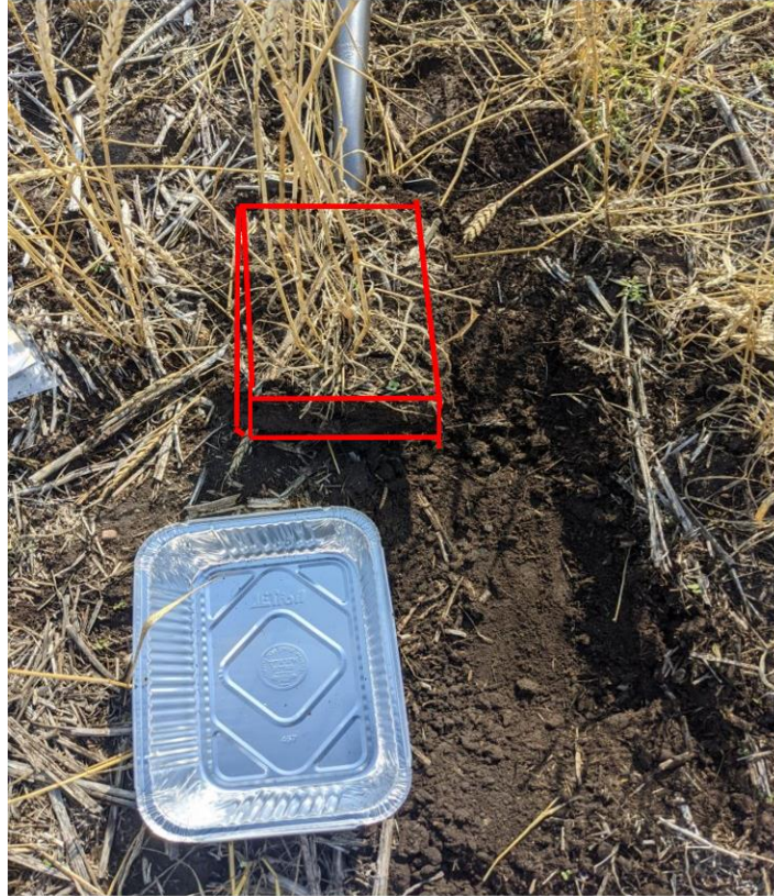
Figure 7. Apparatus used for intact soil slab removal.
